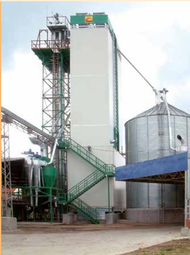
■ Industrial drying ERCL with slow cooling system, with conveyors and cleaners.
